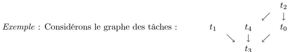
Un ordonnancement possible est  $\sigma(0) = t_2, \sigma(1) = t_1, \sigma(2) = t_4, \sigma(3) = t_0$  et  $\sigma(4) = t_3$ .
